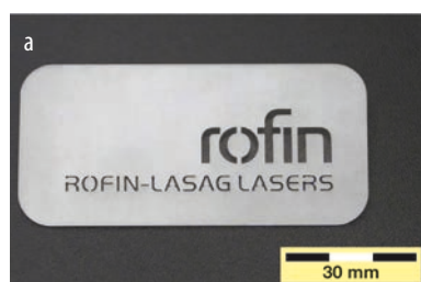
Fig. 4 Exemplary samples of sapphire cut materials. Sapphire wafer cut with fusion cutting process in typical dimensions of a smartphone (a); Edelweiss figure cut from sapphire wafer with fusion cut-
