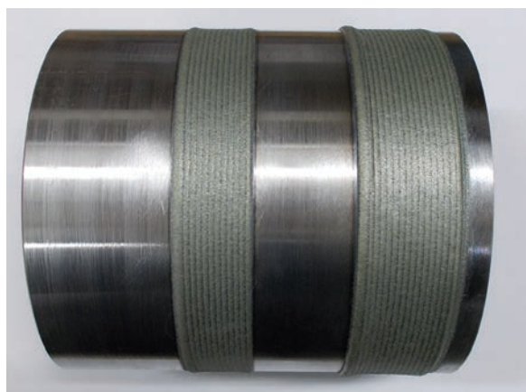
Fig. 4 Thermal laser spraying allows for excellent coating results, not only for the individually dimensioned membrane walls but also for industrial valves, shaft drives or – as shown here – a wear bushing.
