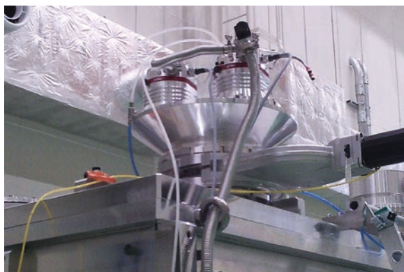
Fig. 2 HiPace turbopumps are installed at European XFEL.
